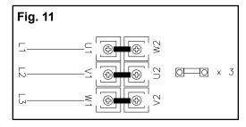
After wiring, make sure the motor is rotating in the proper direction. This is marked on the motor end cover. If the rotation is incorrect, swap the two wires going to the motor terminals, U1 and W1 as shown in paragraph 4.6 . (This does NOT apply to the RSIB 300)
